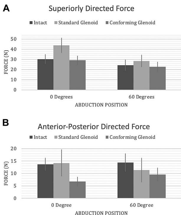
**Figure 4** (A) Average force directed superiorly at 0° and 60° of abduction. The error bars represent the standard error of the mean. (B) Average force directed in anterior or posterior direction at 0° and 60° of abduction. The absolute value of the force was used because both anterior (positive) and posterior (negative) forces are relevant and direction varied by specimen. The error bars represent the standard error of the mean.
