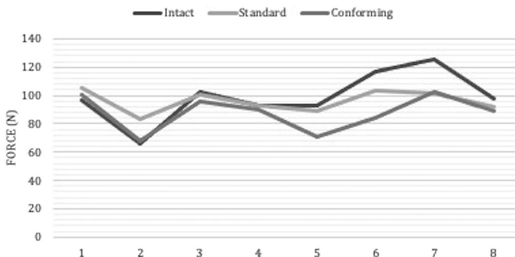
**Figure 5** Maximum force against glenoid (in newtons) for each specimen in each testing condition.
